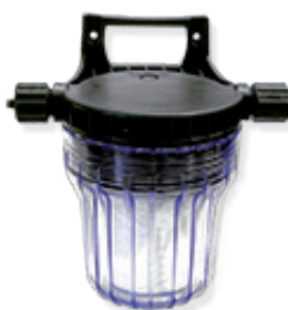
NFIL Filter with cartridge. Washable. PET (60 µ). 6x8 fittings. With LED light sold as option.
