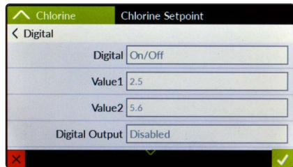
The setpoint for digital outputs can be configured with two working values.
