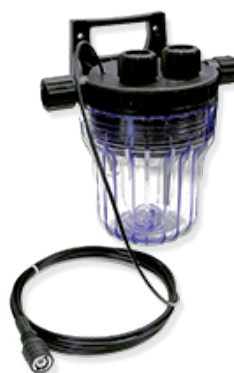
NPED4 Off-line electrode holder for EPH and ERH electrodes. Epoxy \varnothing 12 casing. Max temperature 50° C, max pressure 5bar with flow sensor, N.O. switch, 6x8 fittings. With LED light sold as option.
