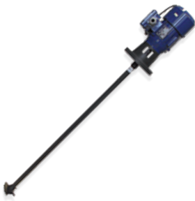
MIXVN/8 High speed mixer 1400 RPM. AISI shaft-PVC coated, different lengths available (630-730-830-930 mm). Marine impeller, diameter 70mm.
