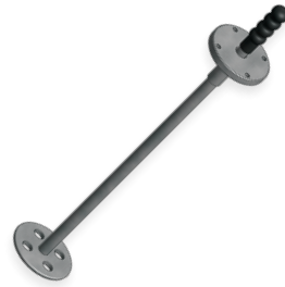
MIX "PISTON" Manual mixer. PVC shaft, different lengths available (500-600 and 700-800 mm). Impeller diameter 130 mm.
