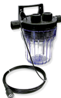
NPED4 Off-line electrode holder for EPH and ERH electrodes. Epoxy Ø12 casing. Max temperature 50° C, max pressure 5bar with flow sensor, N.O. switch, 6x8 fittings. With LED light sold as option.
