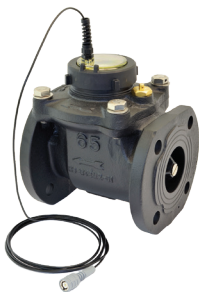
Woltmann dry dial pulse-emitter water meter with Teflon-coated inside and outside.
