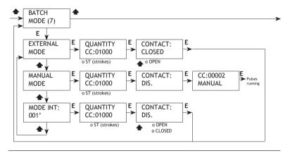
EXTERNAL: an external signal regulates dosing
