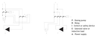
Check the peak absorption. Do not use a motor protector for pumps supplied with 115 or 230 VAC.
