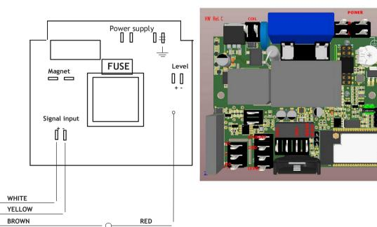
Fig. 39. VMS MF circuit diagram for connection to a pulse water meter with Hall effect
